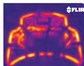
This thermal image shows induction heating at work.
