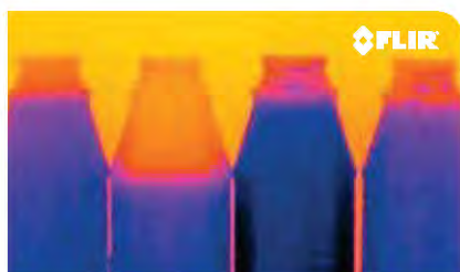
Detecting liquid level in visually opaque bottles.
