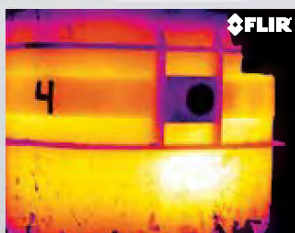
Hot spots on the ladle indicate possible failure.
